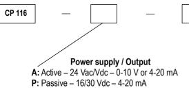
Example: CP 116 - PO Transmitter of atmospheric pressure, passive transmitter 16/30 Vdc, with display
